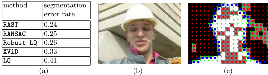
Fig. 4: (a) Average segmentation error rates for the foreman sequence. (b) A frame from the foreman sequence, and (c) a typical segmentation result evaluated using MPEG-4 ground truth segmentation masks. Blue blocks are ignored, red blocks are misclassified.
