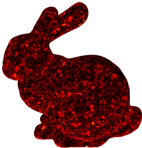
(c) Distance of vertices of original mesh to decimated mesh. The algorithm ran in 1.48 seconds.
