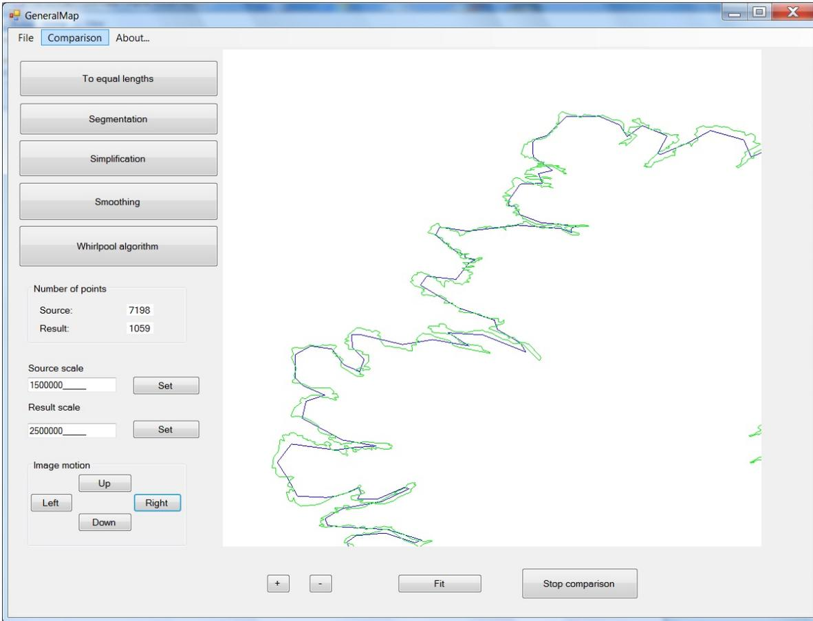
Рис. 2. Result of generalization with our software. The green curve is the given input, and the blue line shows the result of our generalization.
