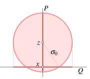
**Fig. 1** A unit Gaussian kernel with center z in  $\mathbb{R}^2$  represented by the disk with radius  $\sigma_0 = 1/\sqrt{2\pi}$ . The lines *P* and *Q* define 1-dimensional sections.
