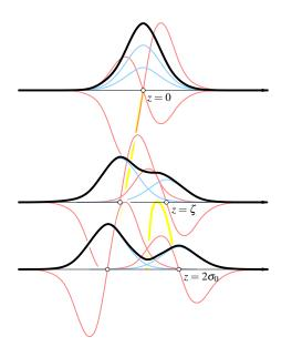
Fig. 3 From top to bottom: the sum of a unit kernel and half a unit kernel. The kernels are blue, their sum is black, their derivatives (plus-minus) are pink, and the trajectories of the critical points, drawn over the interval from 0 to  $2\sigma_0$ , are yellow.
