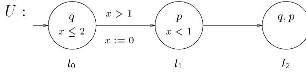
*Example 1.* Consider the TCTL formula  $\psi = z.A(q \vee (1 < z < 3))U(p \wedge q)$  and the linear timed automaton  $\mathcal{U}$  appearing in the figure below.
