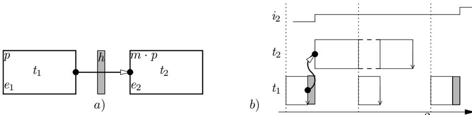
Figure 1. RTW: fast to slow data transfer - (a) task graph; (b) task and signal timeline for  $m = 2$
